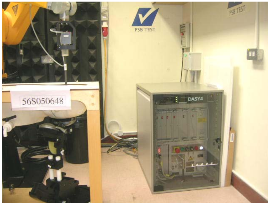
SAR Test Setup (Device at Head Phantom)
