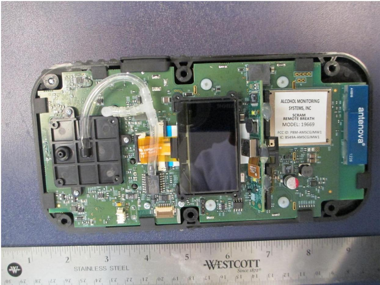
PCBs Inside Remote Breath Housing With Front Removed
