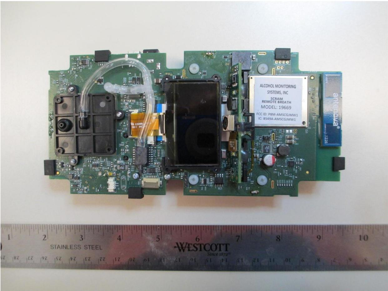
Main Board Top View With Camera Board and Display
