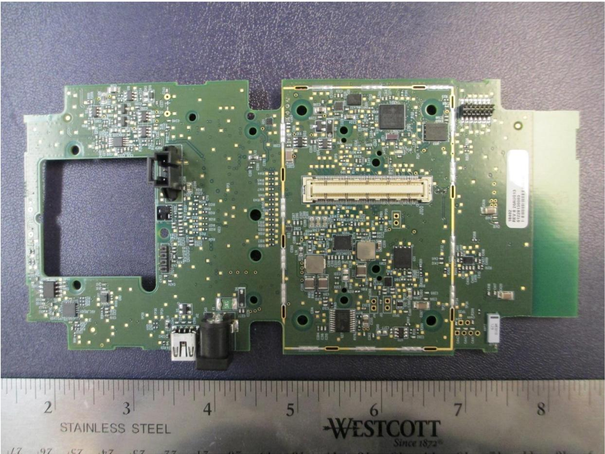
Main Board Bottom View without Processor Board
