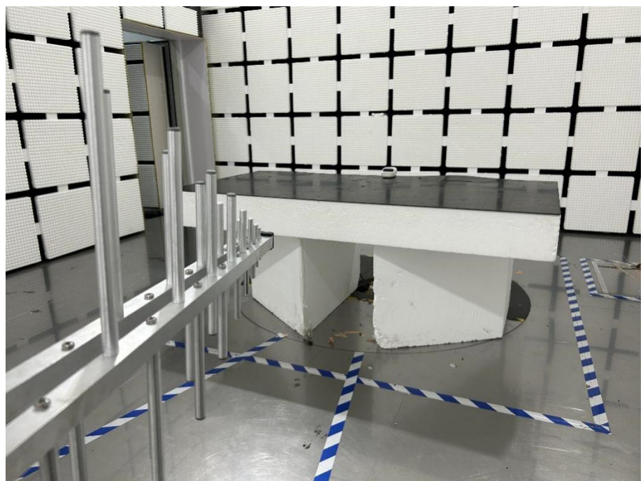
Radiation Emission Test Setup (30MHz to 1GHz)
