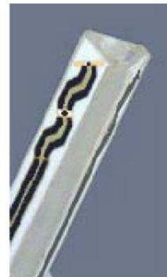
Figure 2.3 Probe Thick-Film Technique
