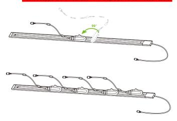
Step 6: First, connect the guideway to the magnetic conductive strip, and then turn on the power to the magnetic conductive strip. Once the guideway is powered up, the device receives energy from Wireless Metal Contacts. This wireless charging technology is similar to the Qi method used in cell phones, ensuring safety and harmless
