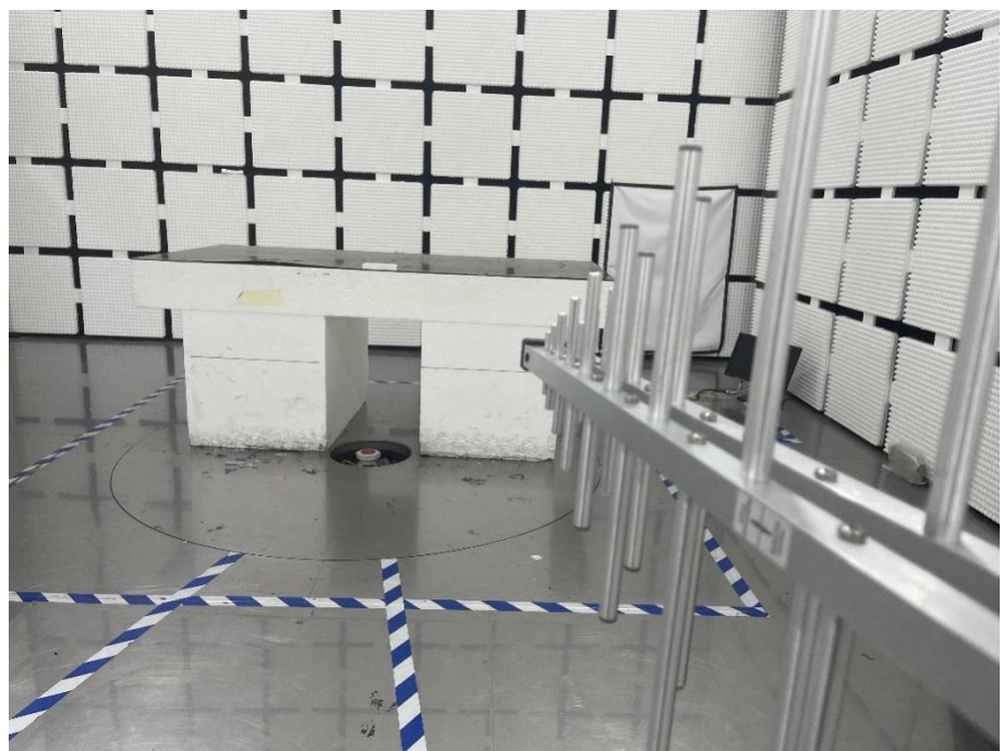
Radiation Emission Test Setup (30MHz to 1GHz)
