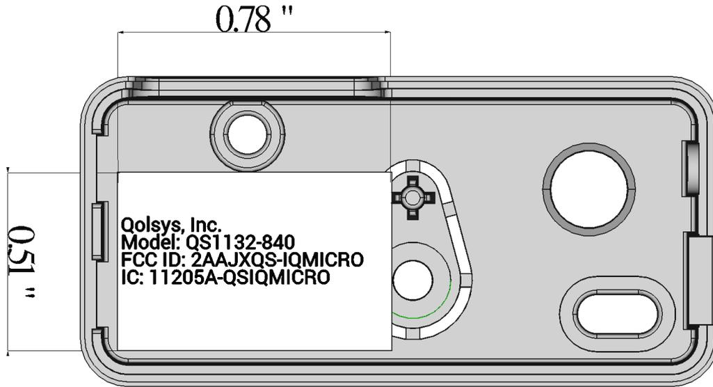
The label is located on the interior of the back plastic. The label will be open to the user and installer when the back plastic is detached from the front.
