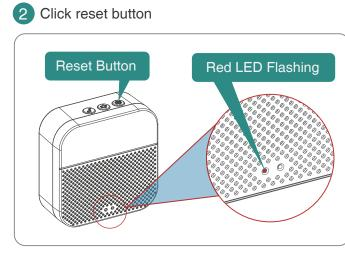
Click on **RESET** only once, and you will see the chime indicator flashing red, indicating that the chime is in pairing mode.
