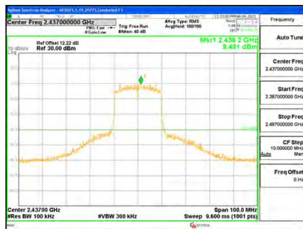
MID CHANNEL REFERENCE LEVEL ANT 3
