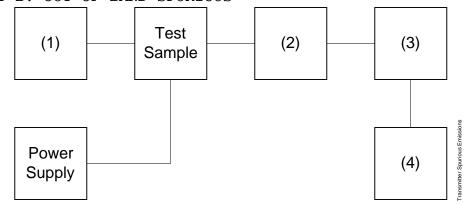
Asset Description s/n (as applicable) (1) AUDIO OSCILLATOR/GENERATOR i00010 HP 204D 1105A04683 i00017 HP 8903A 2216A01753 i00012 HP 3312A 1432A11250 (2) COAXIAL ATTENUATOR i00122 Narda 766-10 7802 i00123 Narda 766-10 7802A i00069 Bird 8329 (30 dB) 1006 i00113 Sierra 661A-3D 1059
