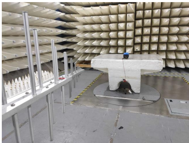
Photograph No.2 Setup for spurious emission field strength measurements in the anechoic chamber above 1000 MHz for Allegro Cellular
