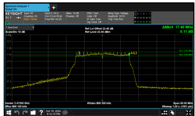
Figure 70 - 802.11n HT20 Maximum 6 dB EBW
