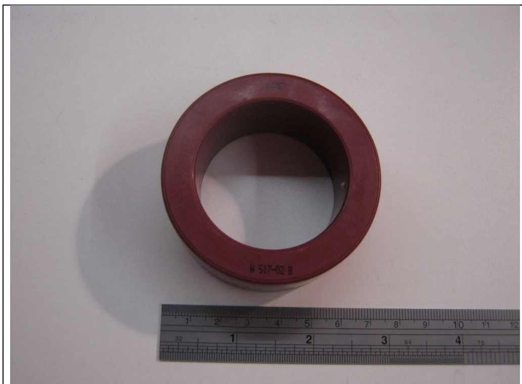
Photograph A3-6: Detail on ferrite VITROPERM 500F, Type 60006-L2063-W157
