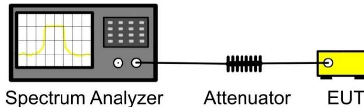
**Block Diagram, Occupied Bandwidth Test Setup**
