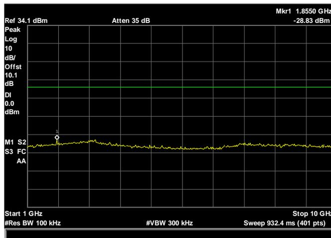
**RF Conducted Spurious Emissions Requirements, 1GHz-10GHz High Channel**
