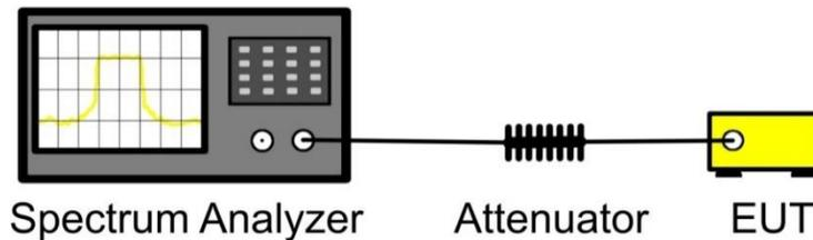
Block Diagram, RF Channel Separation Test Setup
