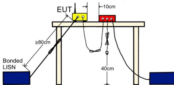
Conducted Emissions Voltage, Test Setup
