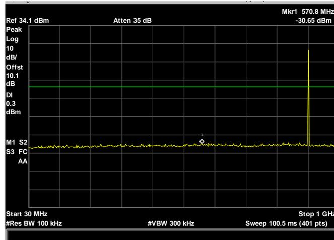
RF Conducted Spurious Emissions Requirements, 30MHz-1GHz Low Channel
