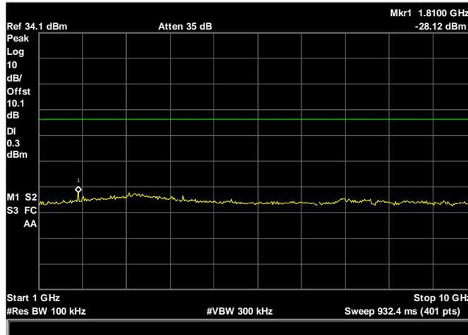
**RF Conducted Spurious Emissions Requirements, 1GHz-10GHz Low Channel**
