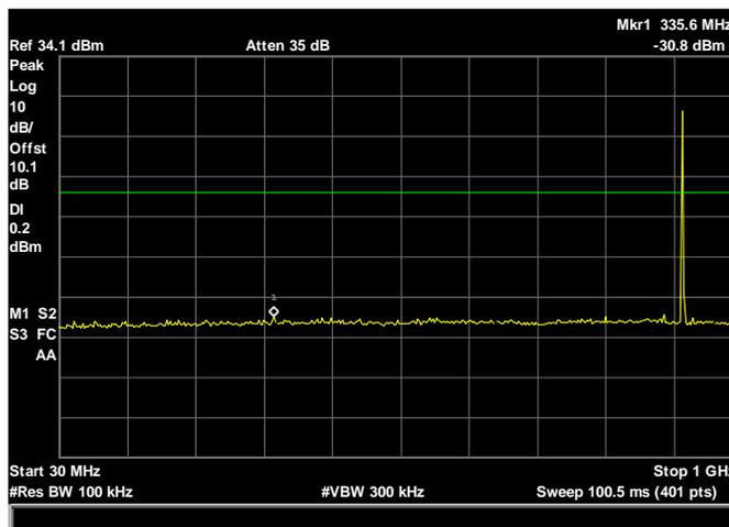
RF Conducted Spurious Emissions Requirements, 30MHz-1GHz Mid Channel
