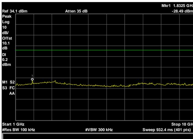
**RF Conducted Spurious Emissions Requirements, 1GHz-10GHz Mid Channel**
