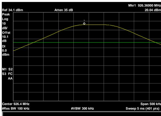
RF Conducted Band Edge, Reference Level High Channel
