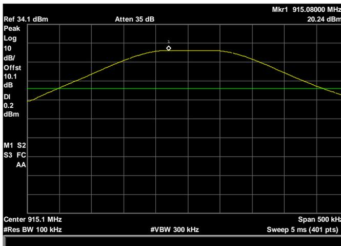
RF Conducted Band Edge, Reference Level Mid Channel
