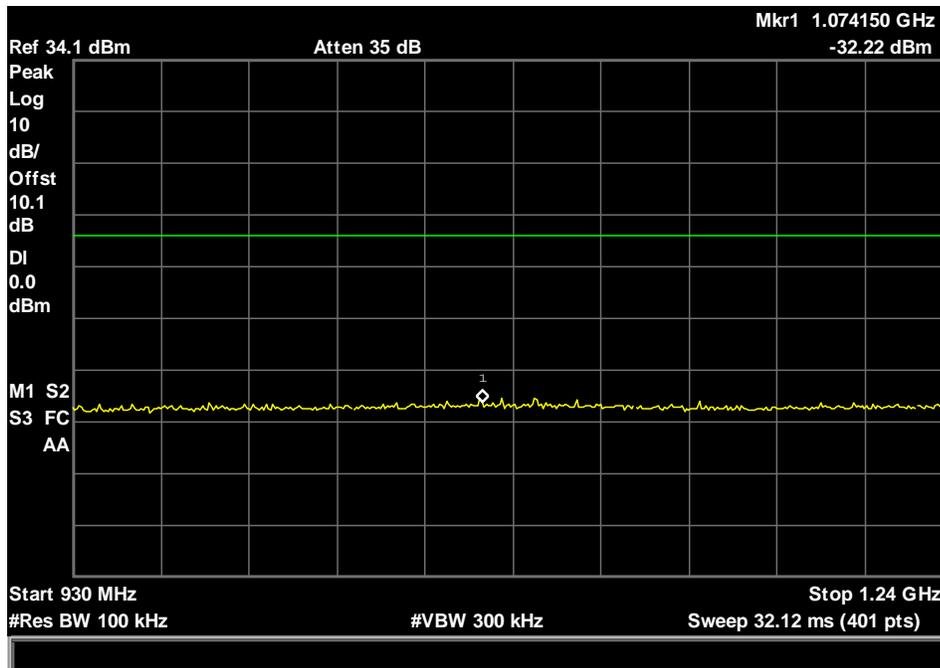
RF Conducted Band Edge, 960MHz-1240MHz Restricted Band, High Channel
