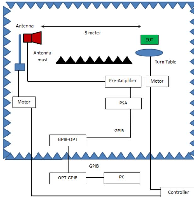
**Radiated Emissions, Above 1GHz, Test Setup**
