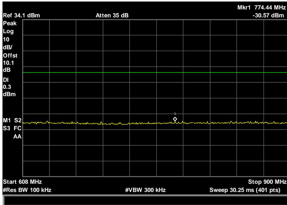
RF Conducted Band Edge, 608MHz-614MHz Restricted Band, Low Channel
