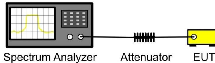
**Block Diagram, Number of RF Channels Test Setup**
