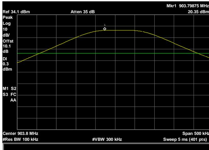
RF Conducted Band Edge, Reference Level Low Channel
