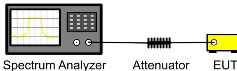
**Block Diagram, Conducted Spurious Emissions Test Setup**
