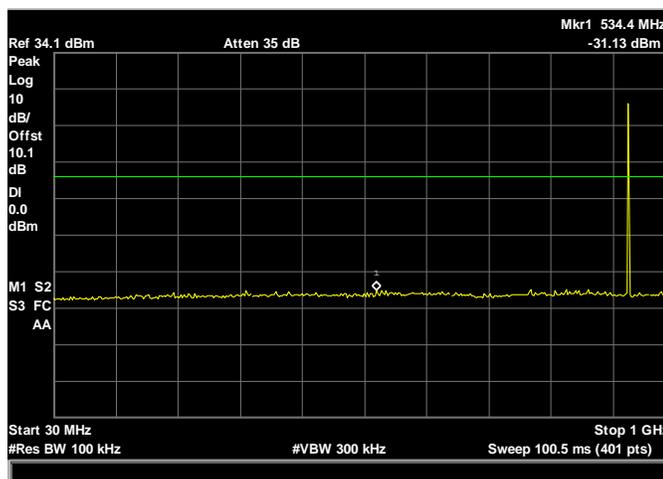
RF Conducted Spurious Emissions Requirements, 30MHz-1GHz High Channel
