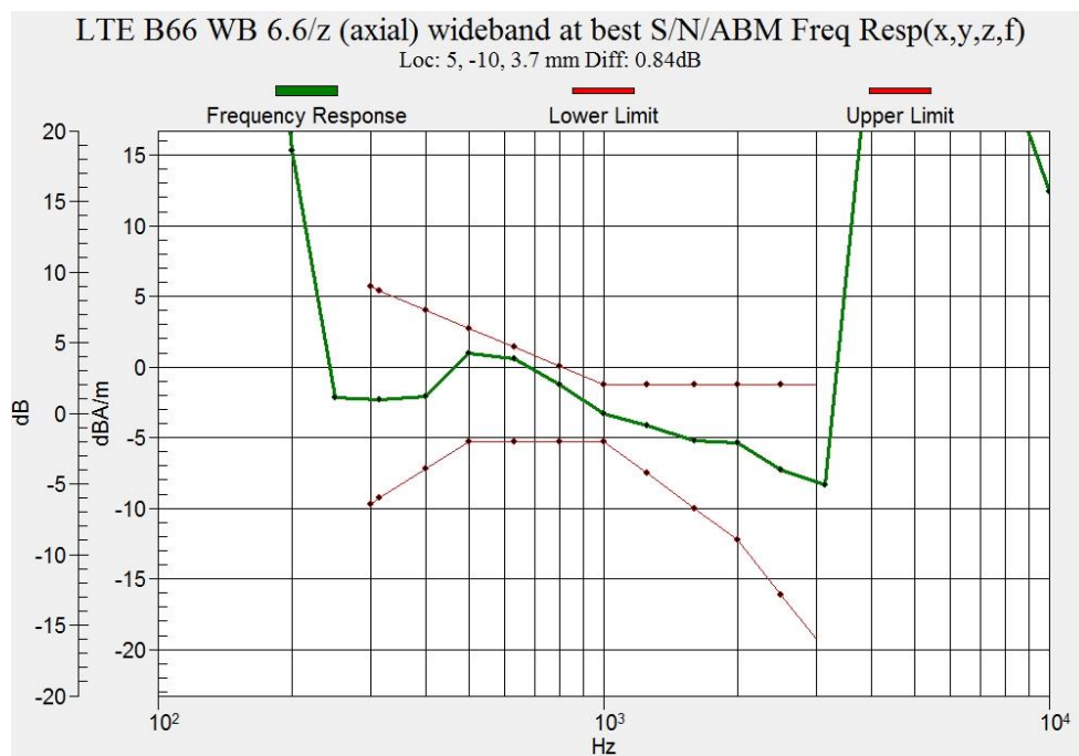
Figure B.22 Frequency Response of LTE Band 66 (Ant.2)
