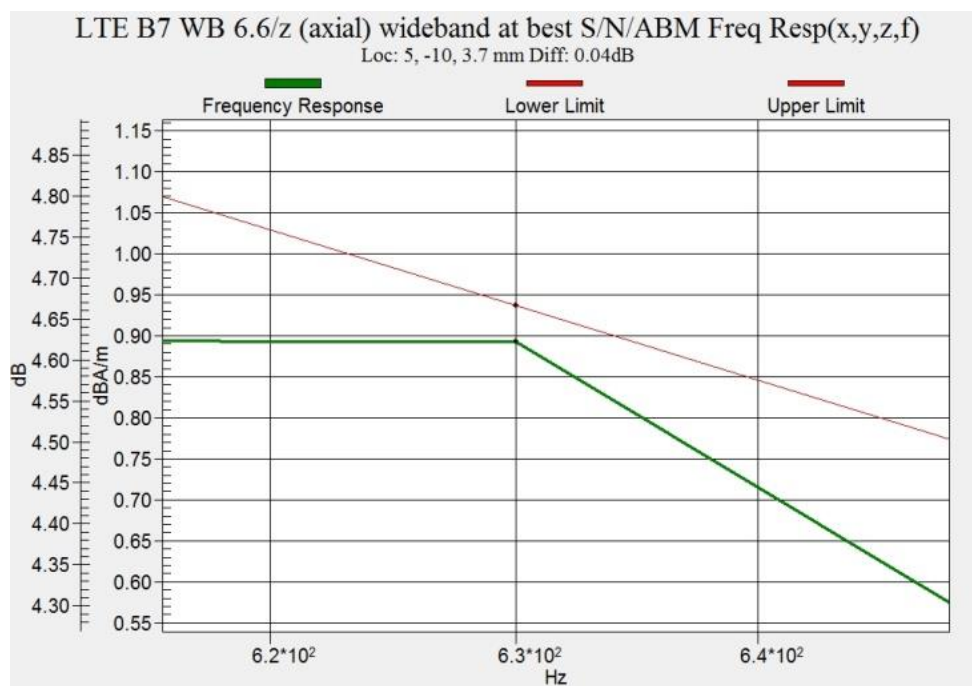
Figure B.12 Frequency Response of LTE Band 7 (Ant.2)
