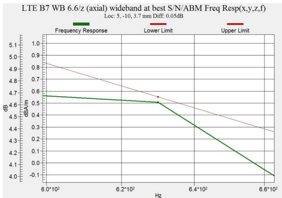
Figure B.11 Frequency Response of LTE Band 7 (Ant.0)
