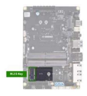
Step 3. Install the new WIFI Module and connect the WIFI antenna cable back to it.
