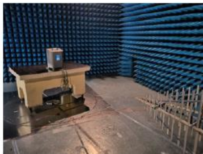
Photo in semi-anechoic chamber – Frequency < 1GHz
