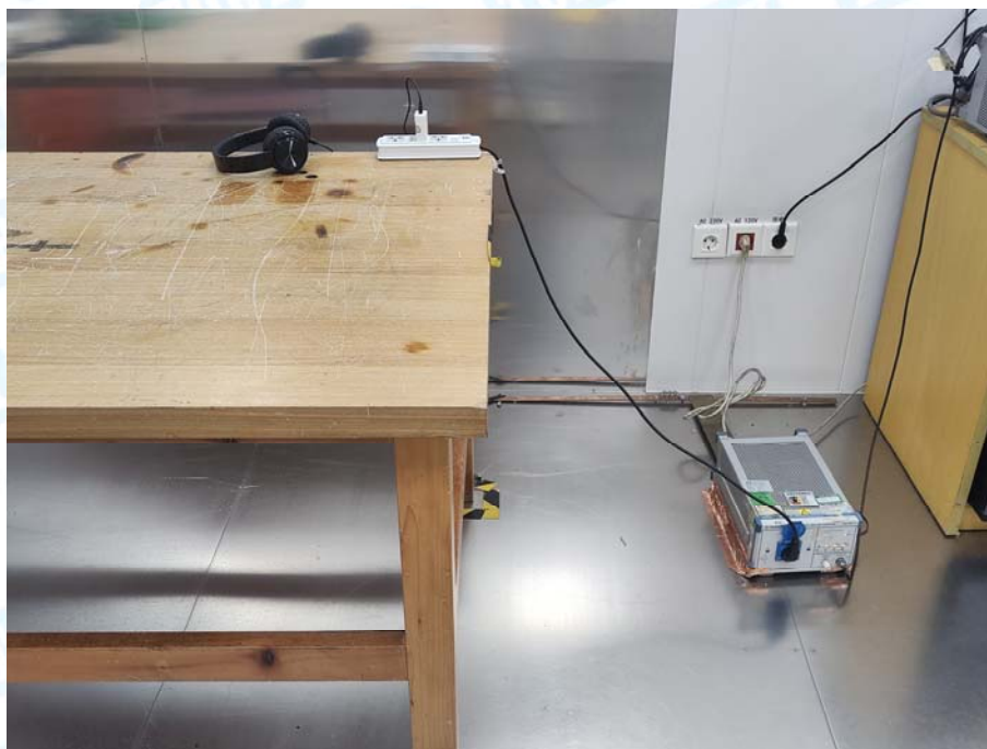
Photo of Setup for Conducted Emission
