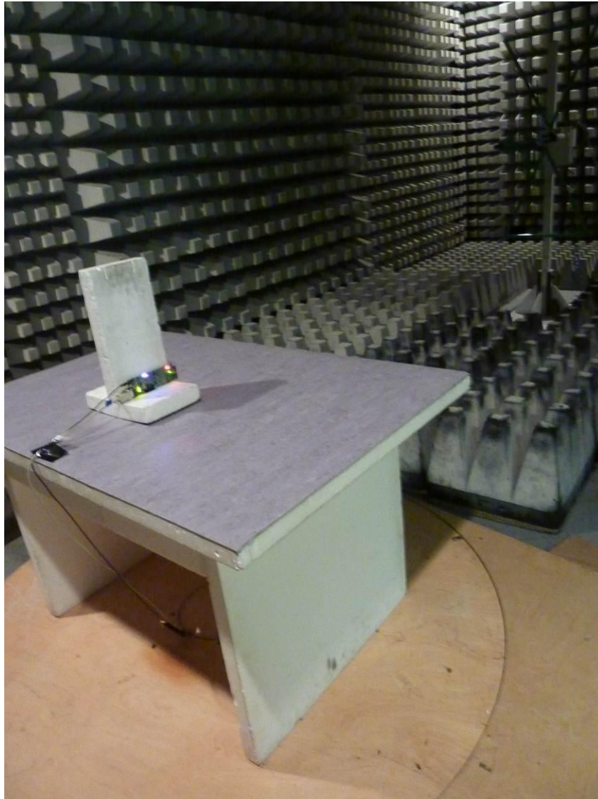
145298_13.jpg: Test setup - Radiated emission (fully anechoic chamber)
