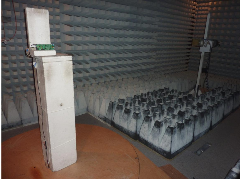
145298_02.jpg: Test setup - Radiated emission (fully anechoic chamber)
