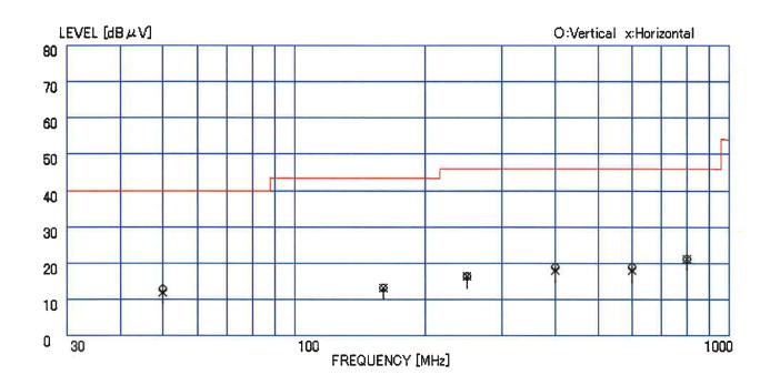
Figure 6.1-1 RFI Field Strength Measurement Results
