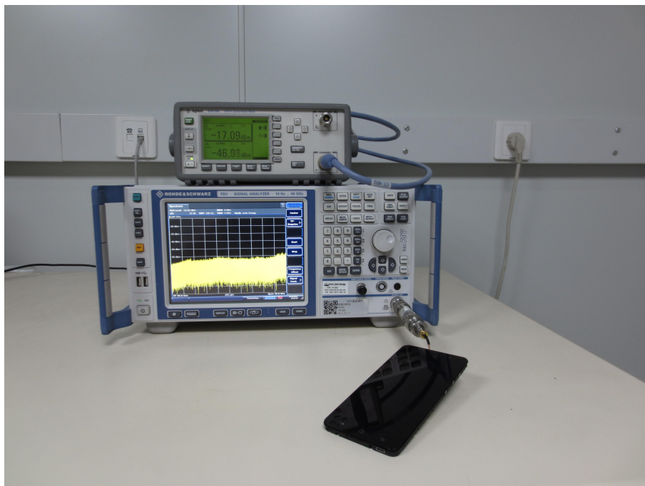
Spurious RF Conducted Emissions Test setup
