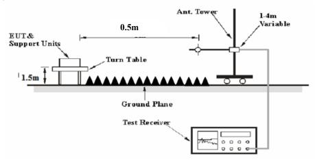
The radiated emission tests were performed in the 3 meters chamber test site, using the setup accordance with the ANSI C63.26-2015. The specification used was the FCC 95.3379 limits.
