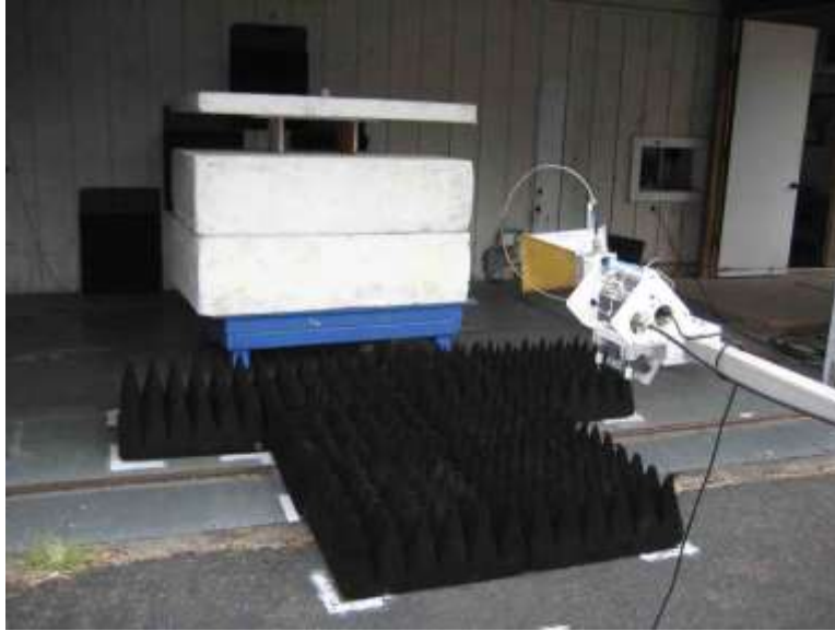
Above 1GHz, Front view, Cone placement
