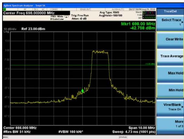
LTE Band 85 16QAM 5MHz CH-Low, 1 RB
