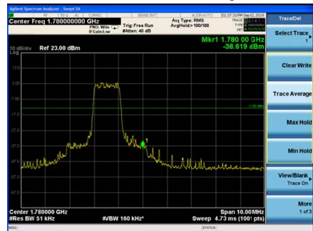
LTE Band 66 QPSK 20MHz CH-High, 1 RB
