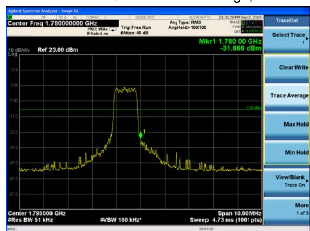
LTE Band 66 16QAM 3MHz CH-High, 1 RB
