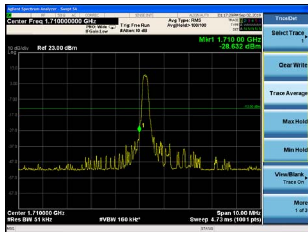
LTE Band 66 16QAM 1.4MHz CH-Low, 100%RB
