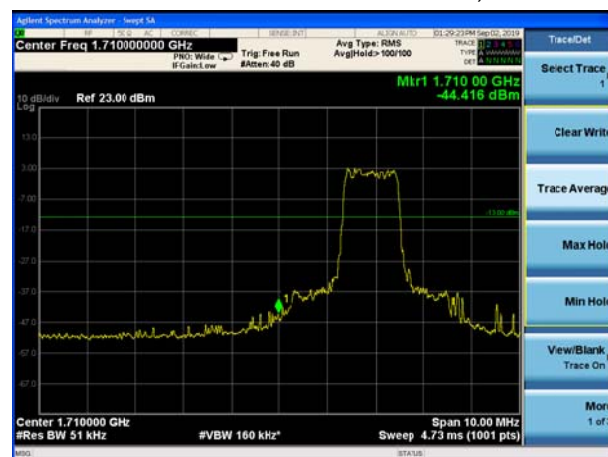
LTE Band 66 QPSK 20MHz CH-Low, 100%RB
