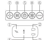
1.DC 5V slot: Use the standard Micro USB V8 charging cable for power charging.
