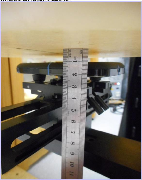
004: Left Hand Side of EUT Facing Phantom at 10mm
