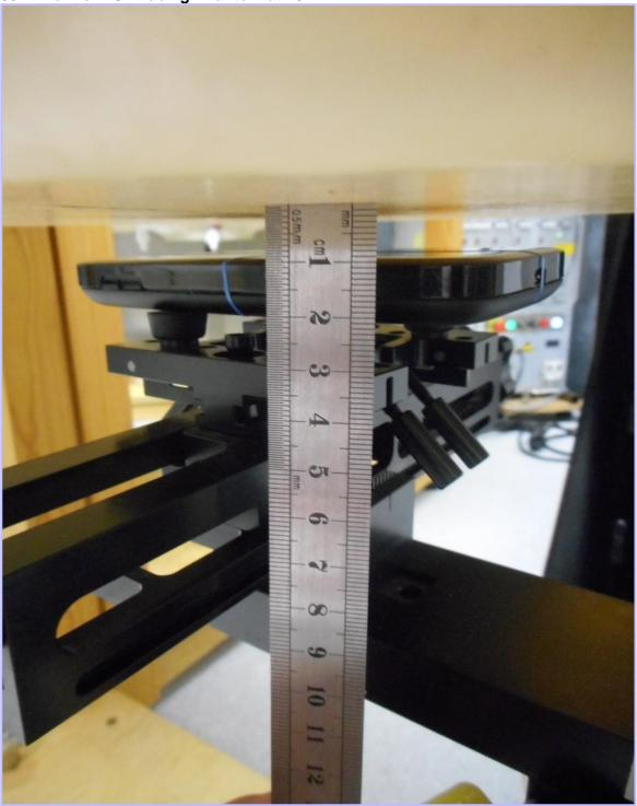
003: Back of EUT Facing Phantom at 10mm
