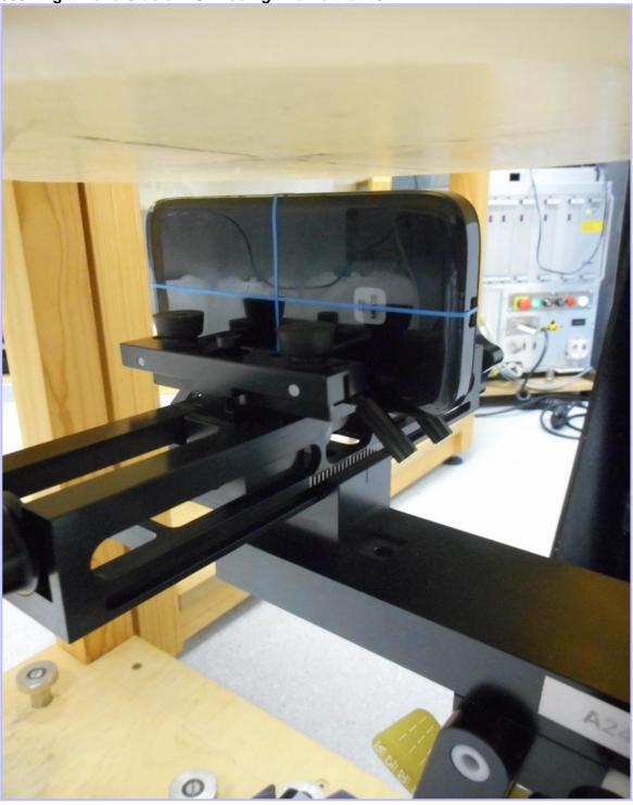
006: Top of EUT Facing Phantom at 10mm
