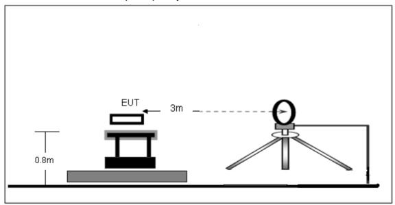
(B) Radiated Emission Test-Up Frequency 30MHz~1GHz
