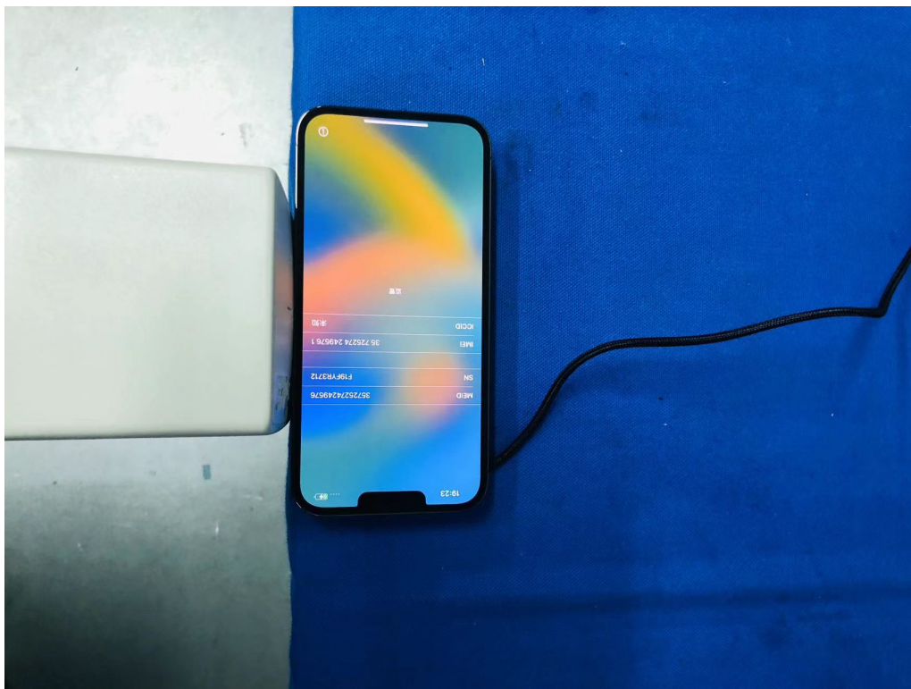
Photograph 4: Set-up for RF Exposure
