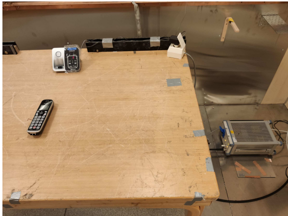
Power-Line Conducted Emissions
