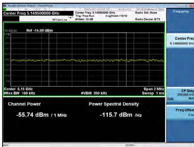
Band Edge-802.11n20 5260 MHz (Limit: -27dBm/MHz eirp)
