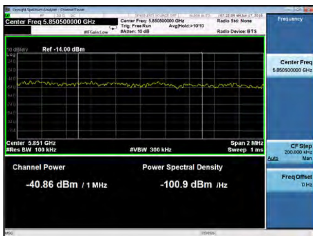
5.8GHz Band Edge-802.11n20 5825 MHz (Limit: -17 eirp)
