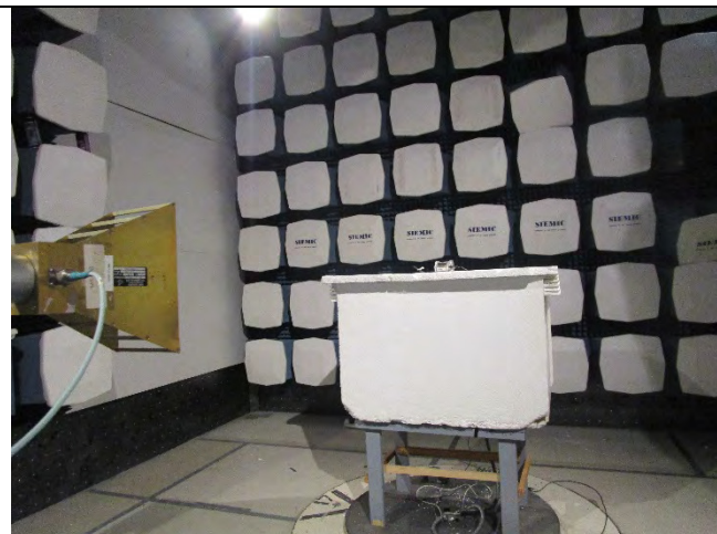
Radiated Emissions (>1GHz) – Front View
