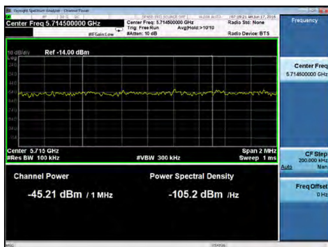
5.8GHz Band Edge-802.11n20 5745 MHz (Limit: -27 eirp)
