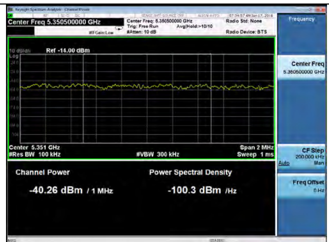
Band Edge-802.11n40 5310 MHz (Limit: -27dBm/MHz eirp)
