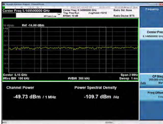
Band Edge-802.11n20 5180 MHz (Limit: -27dBm/MHz eirp)
