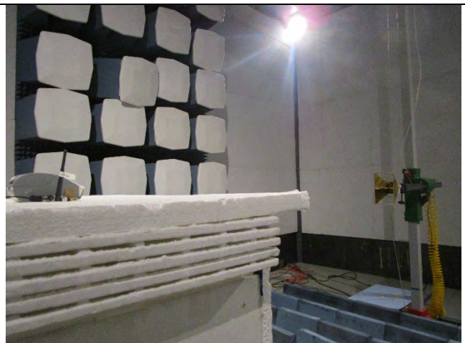
Radiated Emissions (>1GHz) – Rear View
