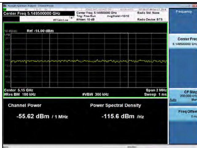
Band Edge-802.11n40 5270 MHz (Limit: -27dBm/MHz eirp)
