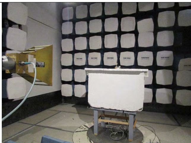
Radiated Emissions (>1GHz) – Front View
