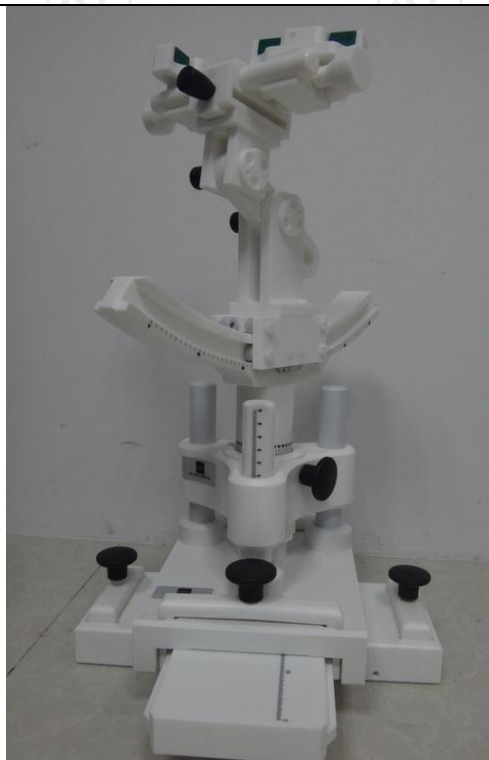
COMOSAR Mobile phone positioning system
