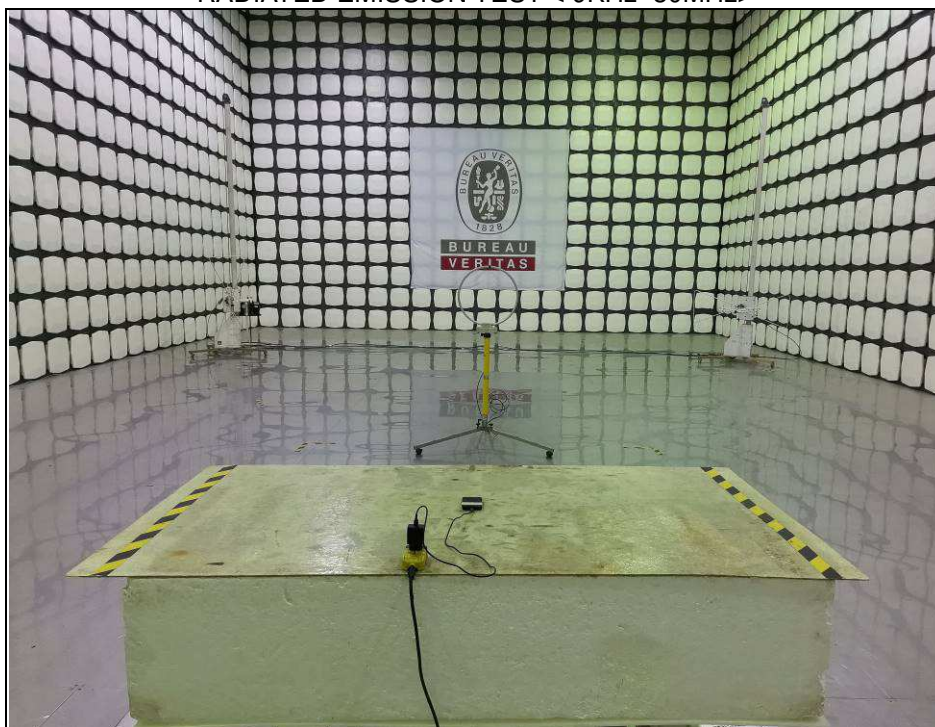
RADIATED EMISSION TEST < 9KHz~30MHz>
