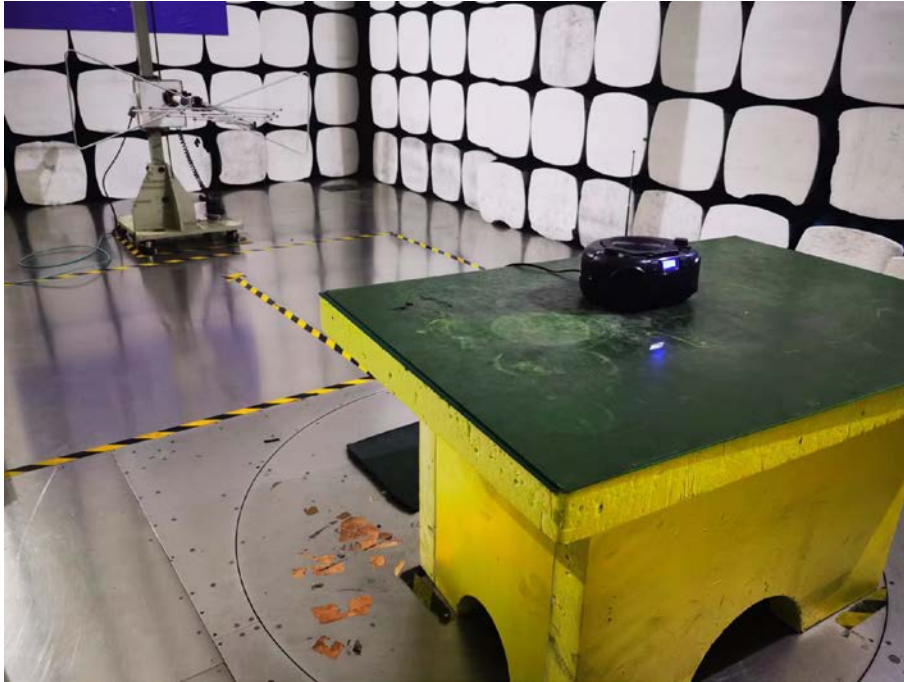
Spurious Emission Test Setup (Below 1GHz)
