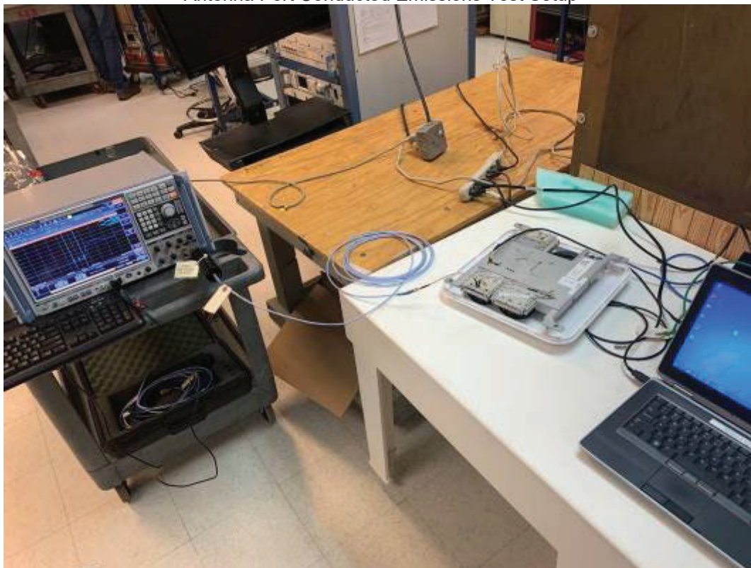
Antenna Port Conducted Emissions Test Setup
