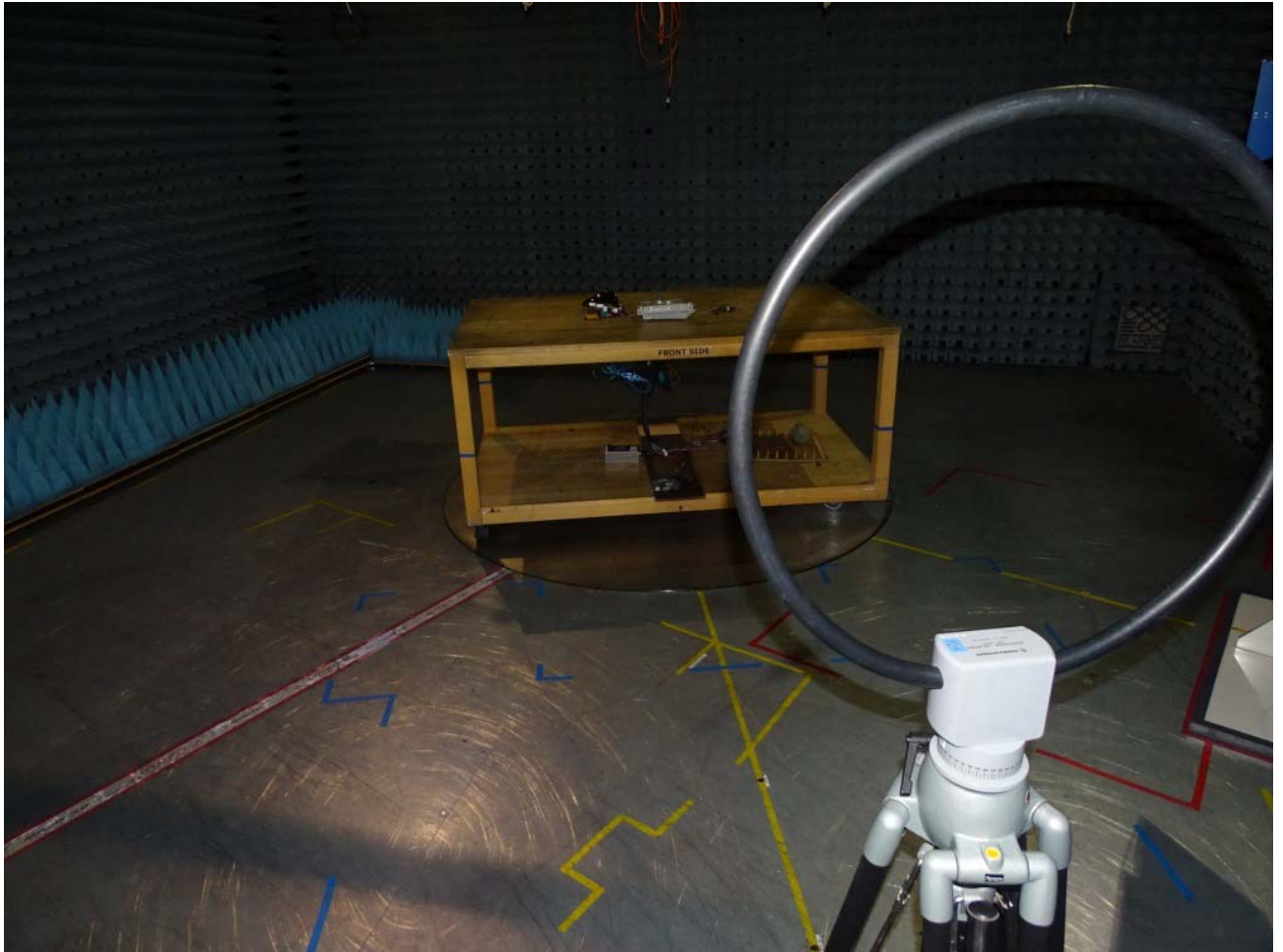
Photo 2: Test setup for radiated measurements below 30 MHz
