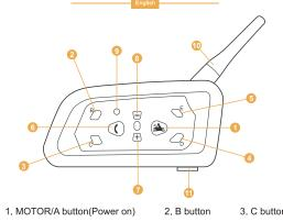
4. D button 5. E button 6. Phone button 8. Volume - 9. Power off 10. Antenna
