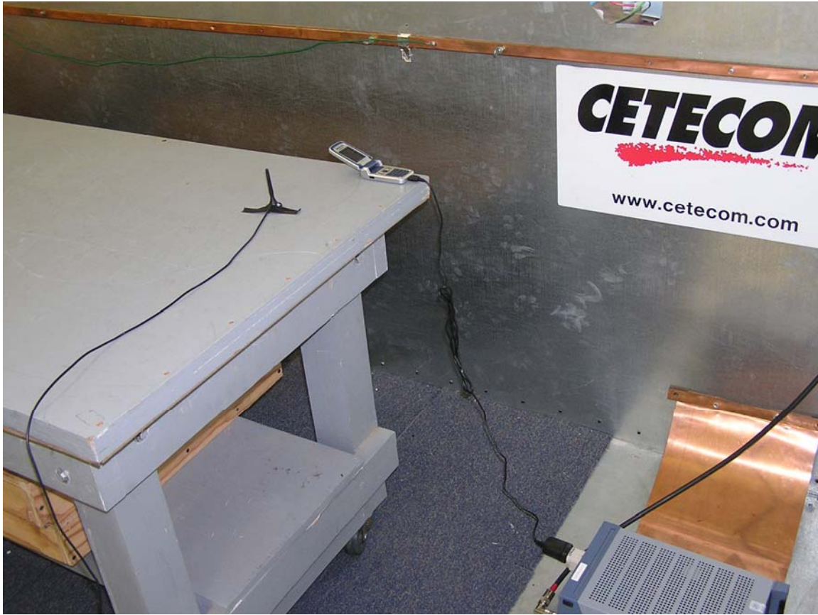
Test setup – AC Line conducted measurements
