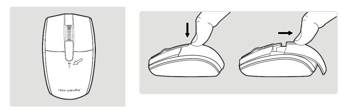
**2** Insert two AAA alkaline batteries with the polarities as shown in the drawing below.
