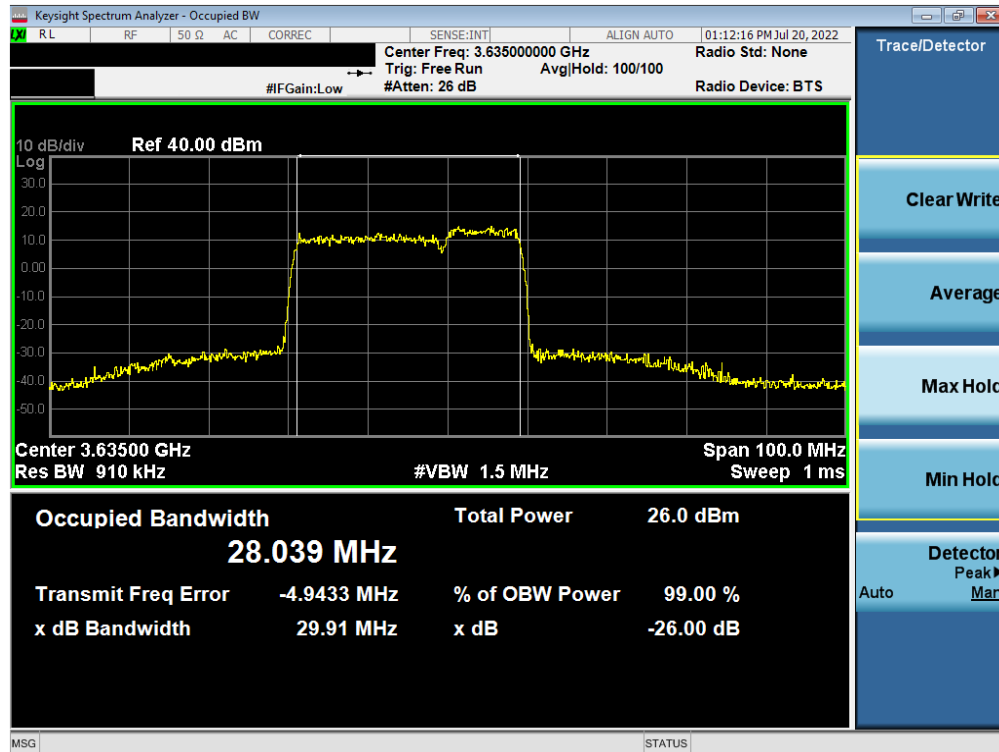
Plot 7-23. Occupied Bandwidth Plot (ULCA Band 48 - 20+10MHz 64-QAM - Full RB Configuration)
