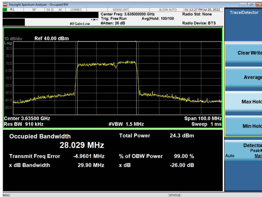
Plot 7-24. Occupied Bandwidth Plot (ULCA Band 48 - 20+10MHz 256-QAM - Full RB Configuration)
