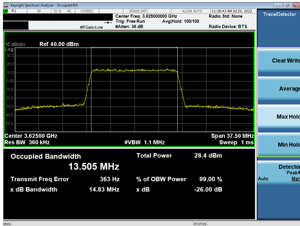
Plot 7-10. Occupied Bandwidth Plot (LTE Band 48 - 15MHz 16-QAM - Full RB Configuration)
