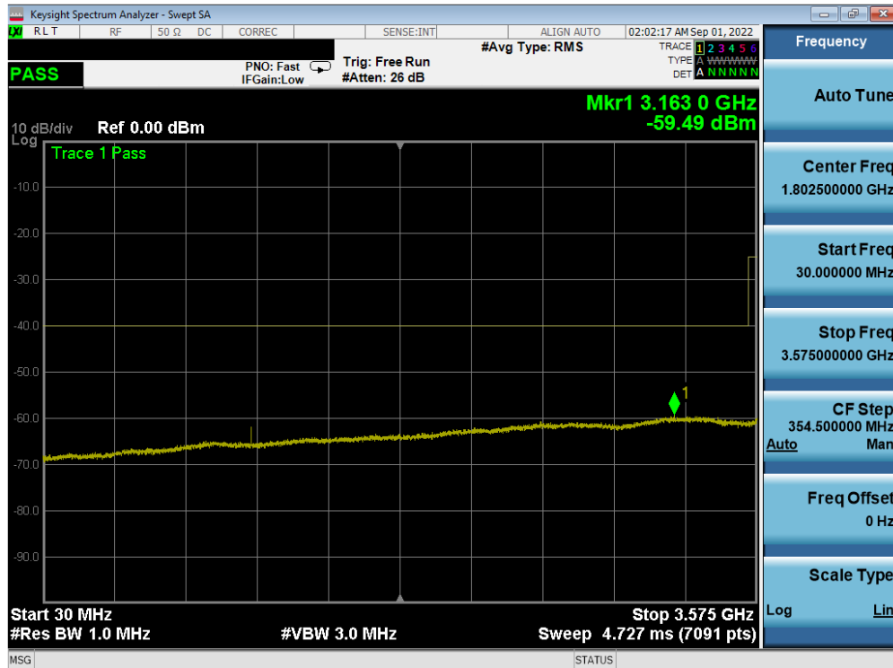
Plot 7-37. Conducted Spurious Plot (LTE Band 48 - 20MHz QPSK - Mid Channel)
