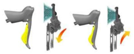
Press the right hand to get bigger button and the small button at the same time, and move the rear dial in the direction of the small tooth. Press the hand change button once, the indicator flashes blue, and then returns to solid on.
