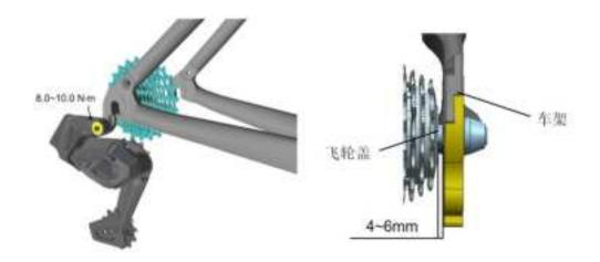
A 5mm Allen wrench is used to attach the transmission to the frame hook, and the appropriate chain is used to alternately pass through the two guide wheels of the transmission. The transmission performance is best when the distance between the inner plane of the chainstay and the outer side of the flywheel minimum gear is maintained at 4-6mm.
