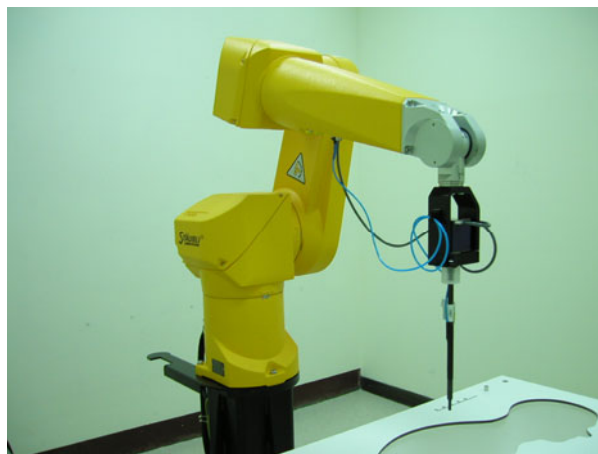
Fig. 5.2 Probe setup on robot
