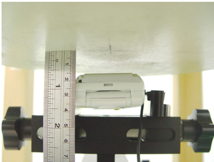
Fig. 9.8 Keypad Down with 1.5cm Gap
