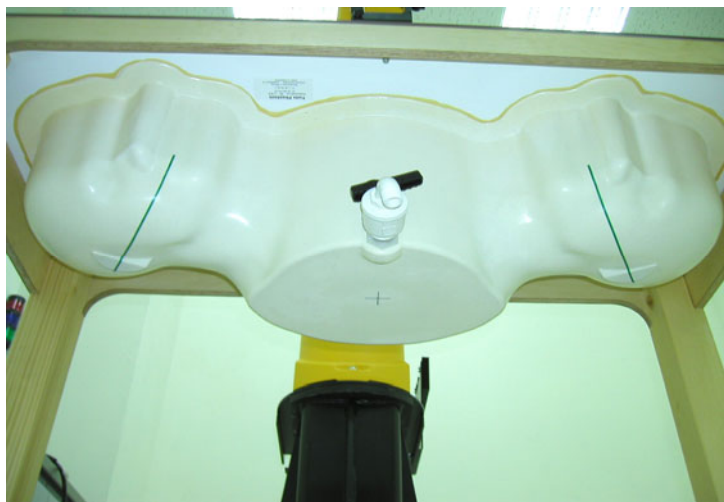
Fig. 5.4 Bottom view of twin phantom
