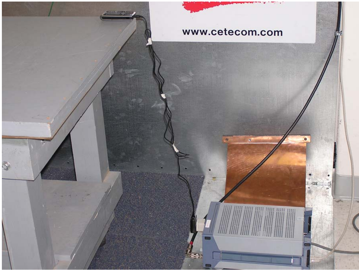
Test setup – AC Line Conducted Emissions
