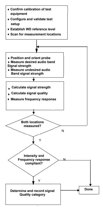
Figure 4-14 C63.19 T-Coil Signal Test Process
