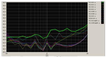
Figure 8-1 **CDMA Audio Band Magnetic Noise**
