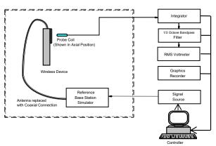
Figure 4-13 **Audio Magnetic Field Test Setup**
