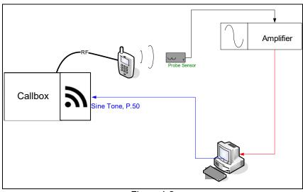
Figure 4-2 **T-Coil Test Setup**
