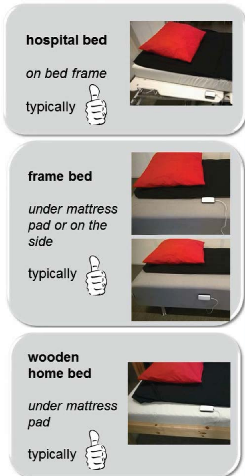
Figure 5. Examples of good SCA11H attachment positions
