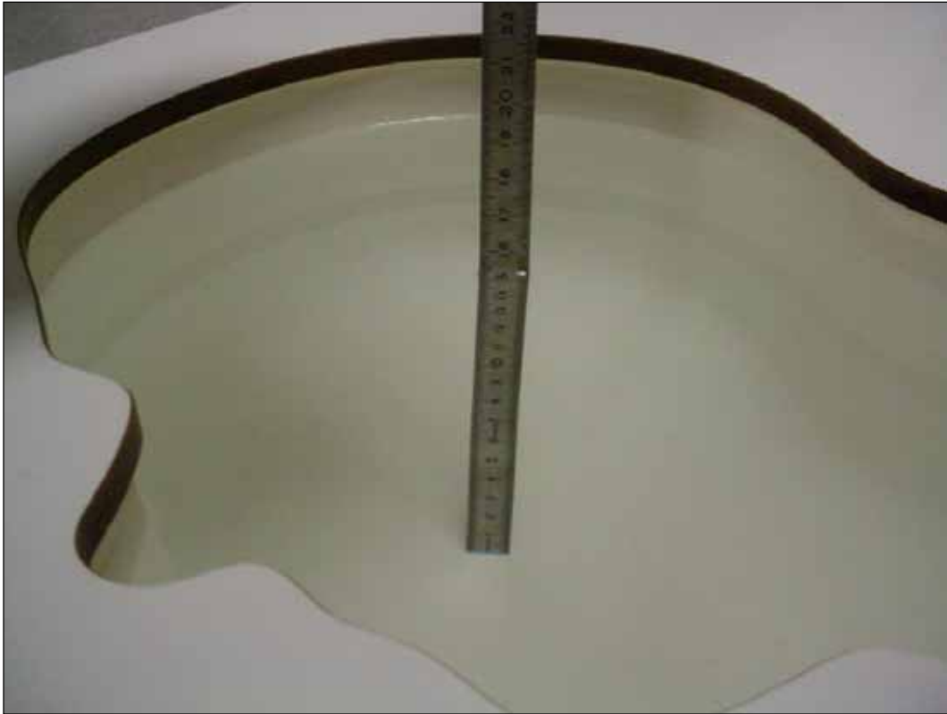
Photo 6: Liquid depth 1750 MHz body simulating liquid
