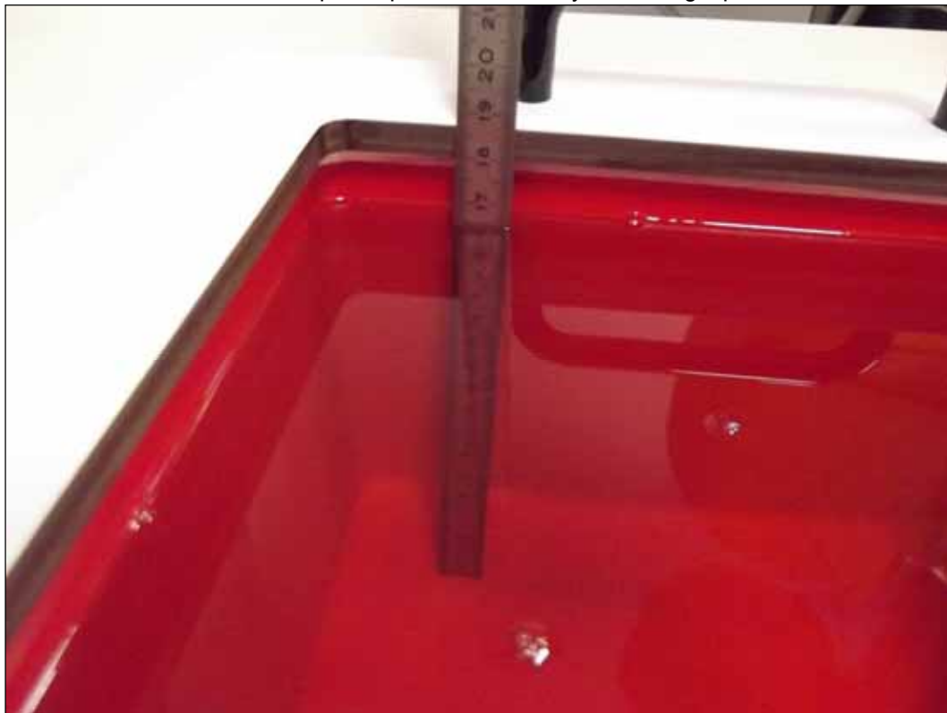
Photo 2: Liquid depth 750 MHz body simulating liquid
