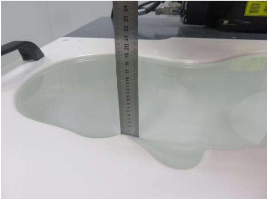
**Photograph of the depth in the Head Phantom (2450MHz, 15.9cm depth)**
