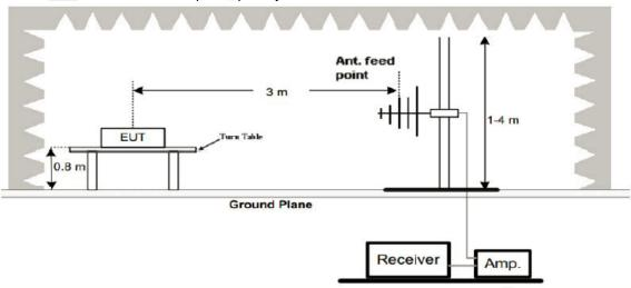
3. Radiated Emission Test-Up Frequency Above 1GHz
