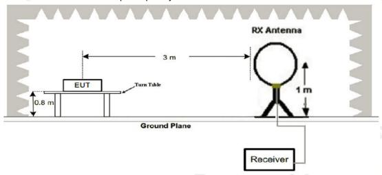
2. Radiated Emission Test-Up Frequency 30MHz~1GHz
