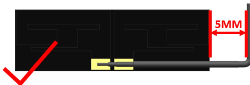
FIGURE 5.2.1 RECOMMENDED CABLE BENDING RANGE
