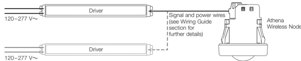
Athena Wireless Node controls up to 5 drivers depending on supply current. IEC 62386 Part 250 requires a minimum guaranteed supply current of 50 mA with a maximum of 250 mA.
