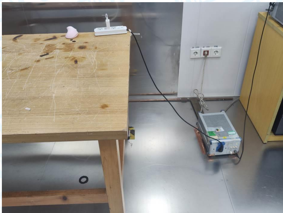
Photo of Setup for Conducted Emission
